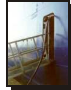
Typical shell door cable entry system
