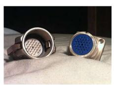
Camlock technology can be used for communications and data circuits. The number of pins and sockets can be varied to between two and seventy, depending on the needs of the customer. Receptacles can be provided with hinged or loose covers and parking receptacles are supplied if required.
