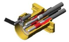
Restrained plugs are used with current ratings from 60 amps to 600 amps, and from 415V to 3.3kV. They should not be fully immersed in water, but operate safely when splashed by waves or drilling fluids. They can be connected by non-electrical personnel and can be designed to different flameproof categories.
